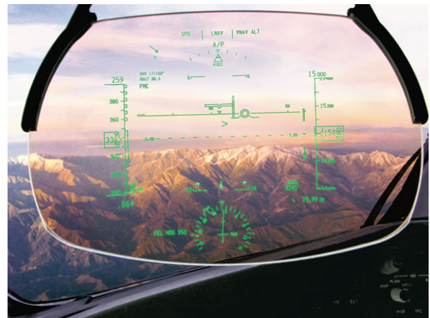
Figure 8: Traditional Head-up Display on a Boeing 787 [6]
