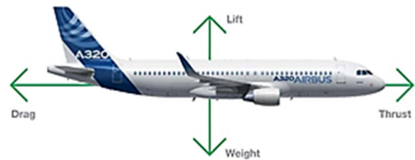
Figure 2: Elementary forces on an airframe
