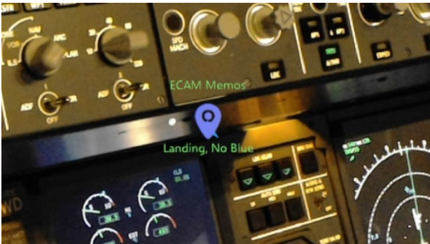
Figure 11. ECAM Memos holographic hint
