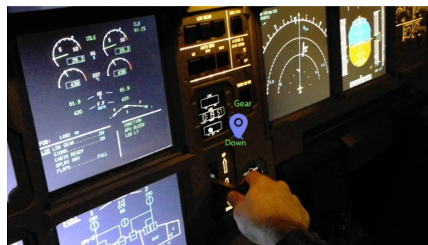
Figure 9. "Gear down" holographic instruction
